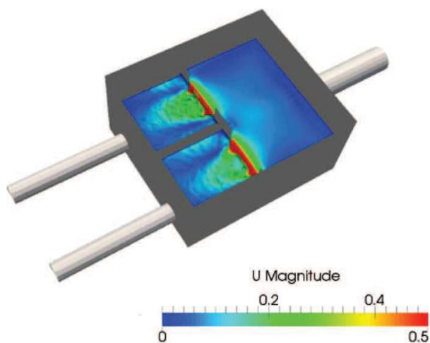
Figure 1 | Surface velocity profile for a flow splitter from open source CFD software (Source: Marques 2015a).
