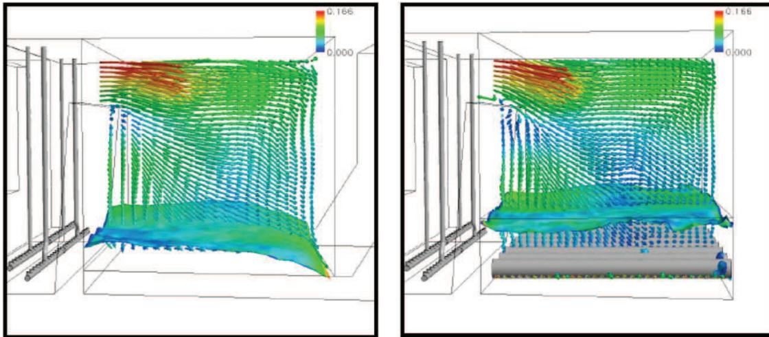
**Figure 4** | CFD Predicted white water level and velocity vector plots in a DAF tank, (left) without and (right) with subnatant tubes (Source: Amato & Wicks 2009).
