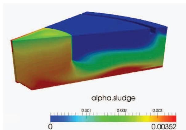
**Figure 3** | Solids profile for a secondary sedimentation CFD simulation developed in open source software (Source: Marques 2015b).
