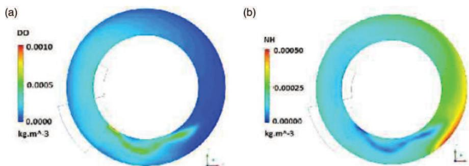
Figure 2 | Oxygen (a) and ammonium (b) concentration plots in a closed-loop reactor (Source: Rehman *et al.* 2014).
